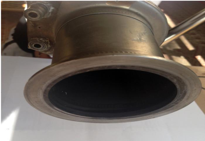
**Figure 1:** Air supply ducting of a B737 aircraft [35].
